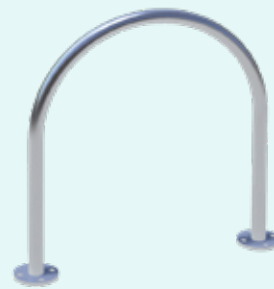
BICYCLE PARKING Name: Semi-Hoop Code: BST03 Dimensions: 845L x 120W x 850H Fixing: Surface mounted Material: Stainless 316 Finish: No.4 Finish (brushed) Supplier: Street Furniture Australia
