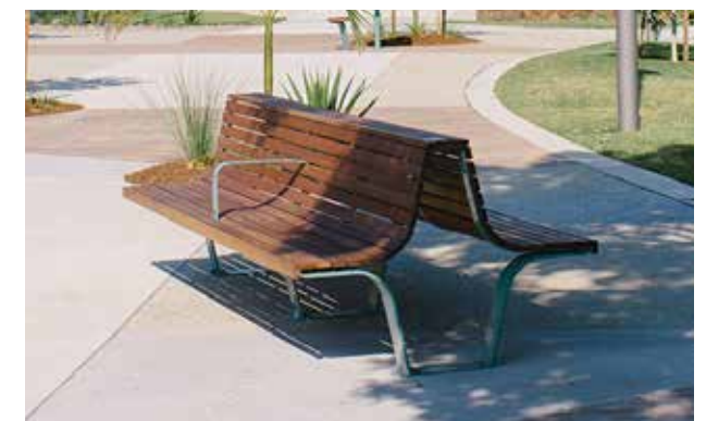
EXAMPLE - TIMBER BENCH SEAT WITH BACK Name: Flip Seat Material: Powdercoated steel, spotted gum slats Supplier: MOS Urban
