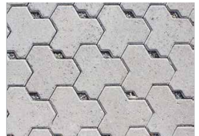
PERMEABLE PAVEMENT - PRE-CAST CONCRETE PAVER Type: EcoTrihex Dimensions: 188L x 92D x 60H Colour: Natural, Charcoal Finish: Shotblast, Honed Supplier: Adbri Masonry
